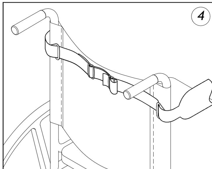
1. ATTACH FLAT-MOUNTS TO WHEELCHAIR BACK CANES USING EXISTING UPHOLSTERY SCREWS OR MOUNTING SCREWS WITH A MINIMUM PULLOUT STRENGTH OF 90kg (200LBS).
