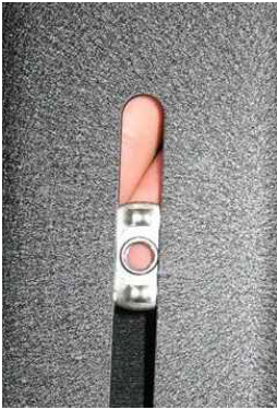
LOWER STRAPS CAN BE FITTED TO EXISTING SLOTS USING WELD NUTS
