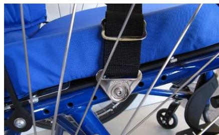
Direct mount\* on tube with threaded holes
