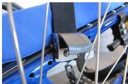
Direct mount\* on tube with threaded holes
