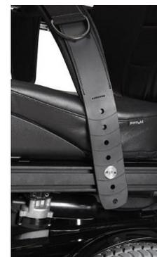
With Evoflex® Hip Belt, using HKA6-12MM bolt and washer, and Evoflex® wave spring washer and flange nut
