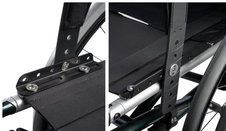
Mount on upholstery strip with Evoflex® Hip Belt, using Evoflex® M6 X 8mm screw, wave spring washer, and flange nut
