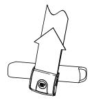
BELT POSITION AND LENGTH CAN BE ADJUSTED AFTER INSTALLING CINCH-MOUNT TO TUBING
